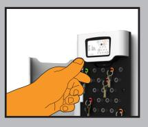
All keys and keysets are individually locked by the Traka 21 unit. Green LEDs indicate those keys to which this user has access. The user cannot remove keys highlighted by the Red LEDs which remain locked in place.
